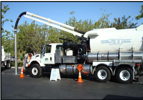
TCWD'S Vactor Truck is routinely used to clean District sewer main lines as preventative maintenance.
