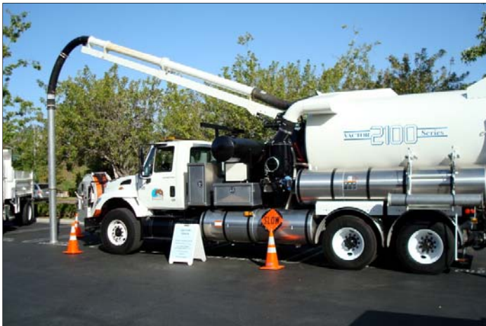
TCWD'S Vactor Truck is routinely used to clean the District's sewer main lines as preventative maintenance.
